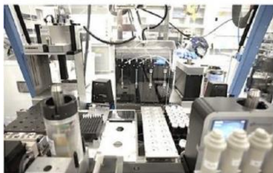
Figure 2-2: Electronic polymer synthesis platform of Polybot, an AI-integrated robotic synthesis laboratory ( Chem. Mater. 35 , 3046 [2023]).
